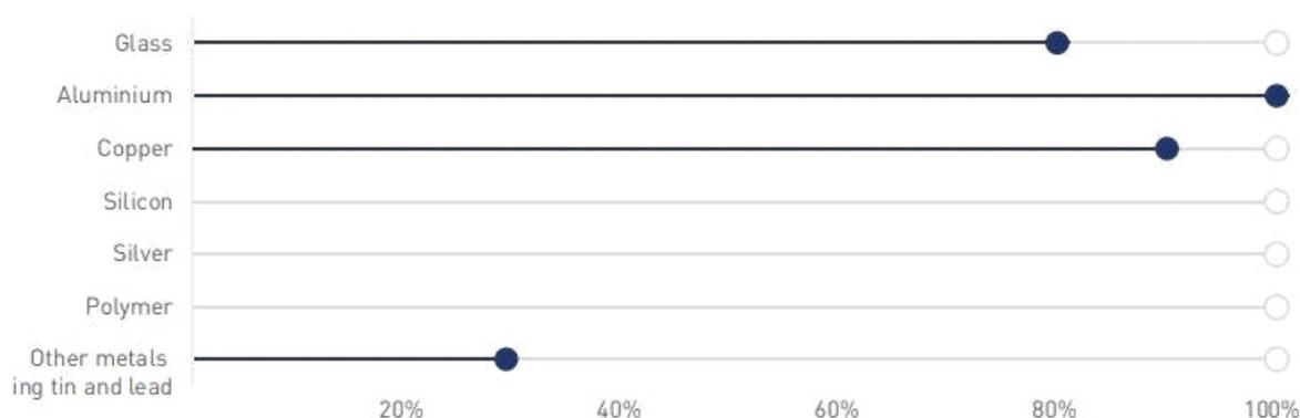
Fig: 7 Raw material recovered by conventional recycling (Source: BRIDGE TO INDIA)
