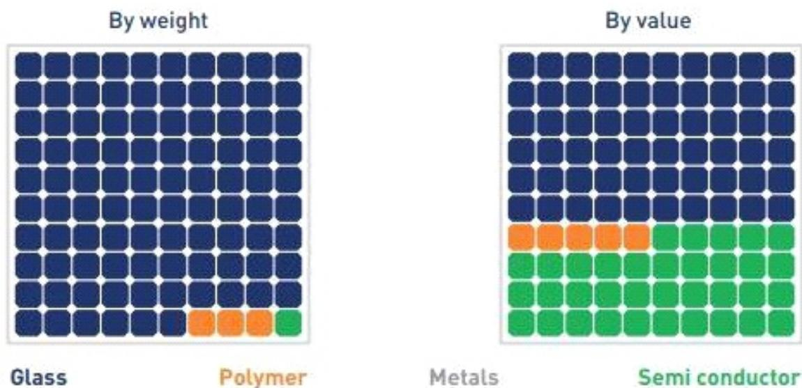
Fig: 6 Material Composition of thin-film solar modules (Source: IRENA and BRIDGETO INDIA)
