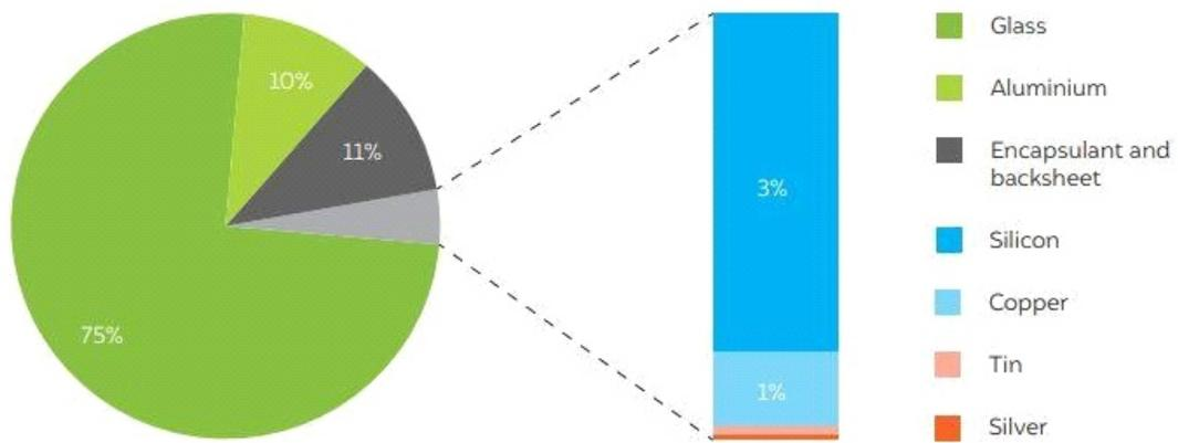
Fig: 3 Composition of crystalline silicon module (Source: European Commission DG ENV 2011 and CEEW)
