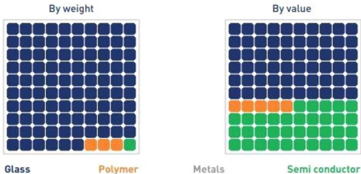
Fig: 6 Material Composition of thin-film solar modules (Source: IRENA and BRIDGETO INDIA)
