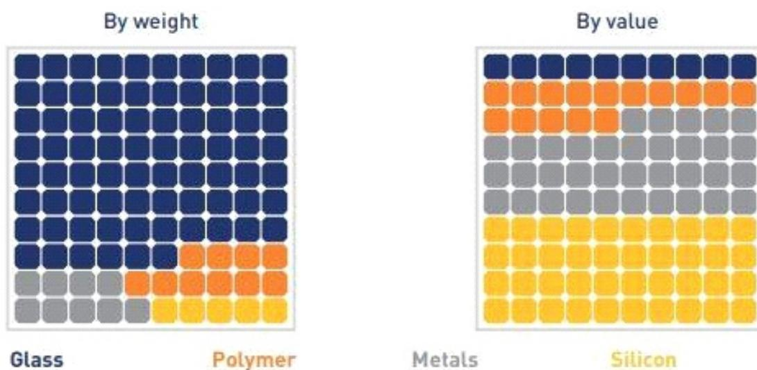
Fig: 5 Material Composition of C-Si solar modules (Source: IRENA and BRIDGETO INDIA)
