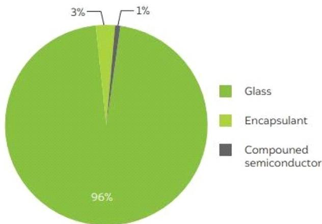
Fig: 4 Composition of the CdTe thin film module (Source: IRENA and IEA-PVPS 2016)
